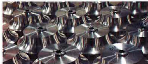
Above, a batch of newly machined impeller blanks.
