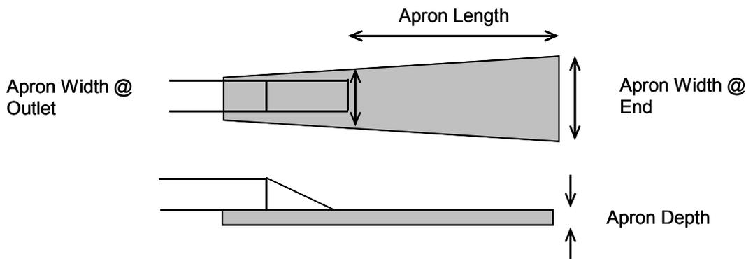
Apron Width at Outlet: Width = 3\*pipe dia. (or width of channel)
