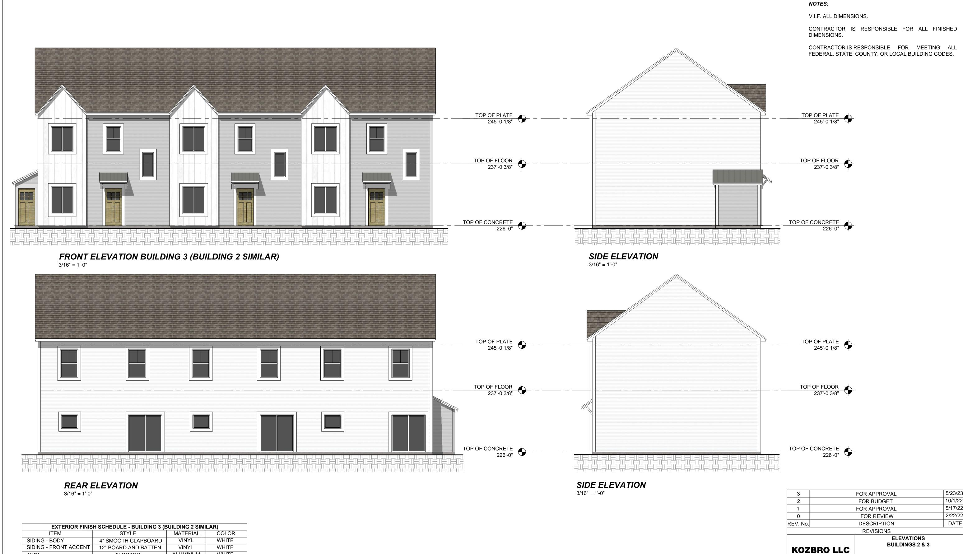
WHITE 6" BOARD ALUMINUM ROOFING - GABLE ARCHITECTURAL SHINGLE CHARCOAL ASPHALT SOFFIT - GABLE 12" SMOOTH VENTED VINYL WHITE ROOFING - SHED STANDING SEAM METAL DARK GRAY WINDOW - FRAME **VARIOUS** VINYL WHITE COMPOSITE LIGHT WOOD DOOR MODERN FARMHOUSE CEMENT DARK GRAY FOUNDATION FASCIA BOARD
