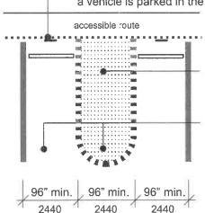
**96" min. width access aisle**, level (max. slope 1:50 in all directions), located beside the van parking space
