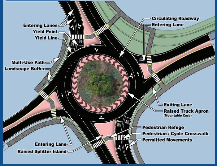
Modern Roundabouts are a circular intersection design with traffic control features that control driver behavior. These features include entering traffic yield signs, chanalized approaches and design that helps to insure relatively low and safe travel speeds.
